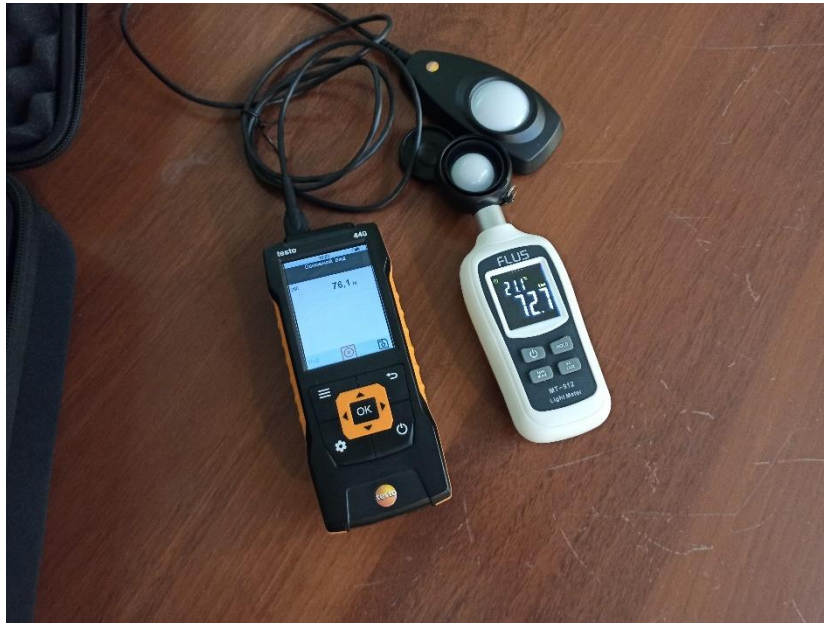
Fig 2.10. Devices used for the survey left -Testo 440, right Flus MT-91
