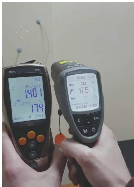
Fig. 5.18 Comparison of measurement readings with pyrometer and device
