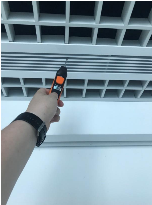
Fig. 4.27. Application of Testo 915i to measure substance temperature
