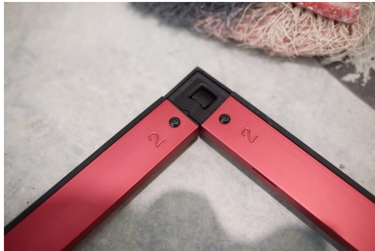
Fig.6.11 Connecting the air door grooves, number to number
