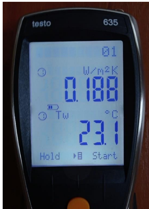
Fig. 5.21 Calculation of the actual thermal conductivity of the envelope by a device
