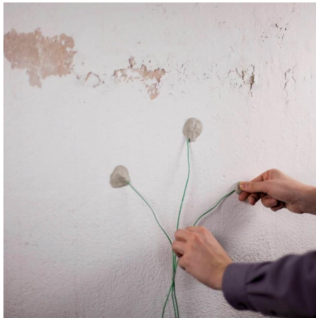
Fig 5.16 Example of fixing a 3-phase probe
