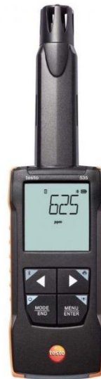
Fig. 1.4. Testo 535 device to measure microclimate parameters
