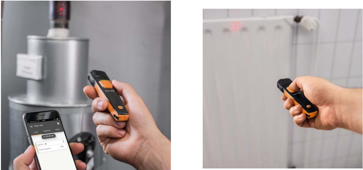
Fig. 4.30. Non-contact surface temperature measurement with the mini pyrometer Testo 805i device
