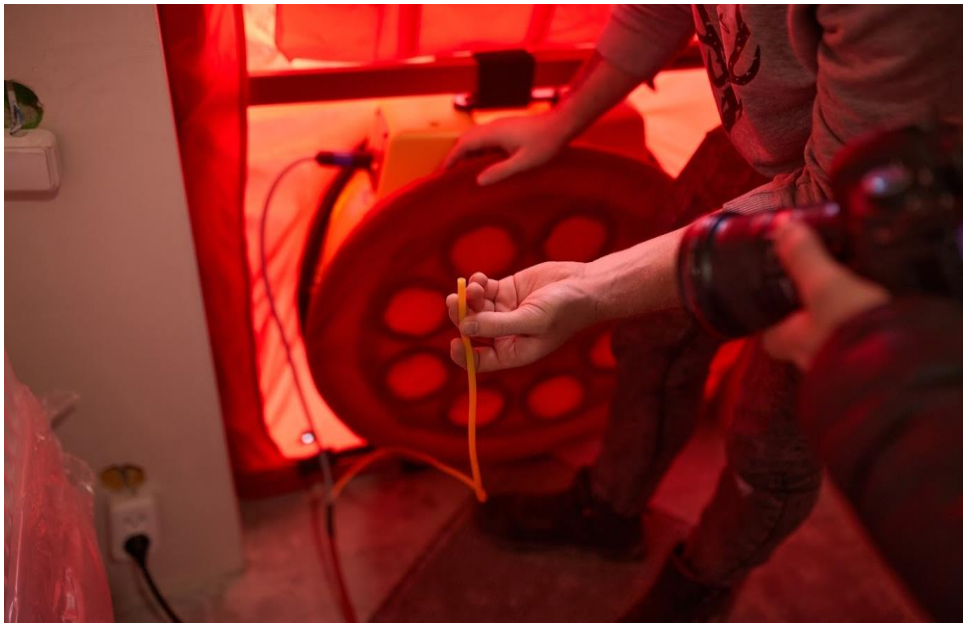
Fig. 17 Installation of the yellow cable in the fan opening
