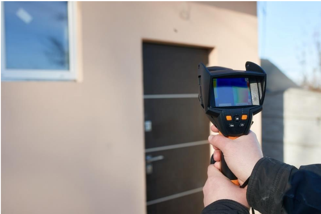
Fig.5.15 Using thermal imaging device to find problem areas in the building insulation
