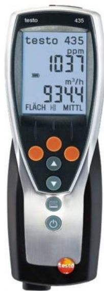
Fig. 4.18. Multifunctional device - Testo 435
