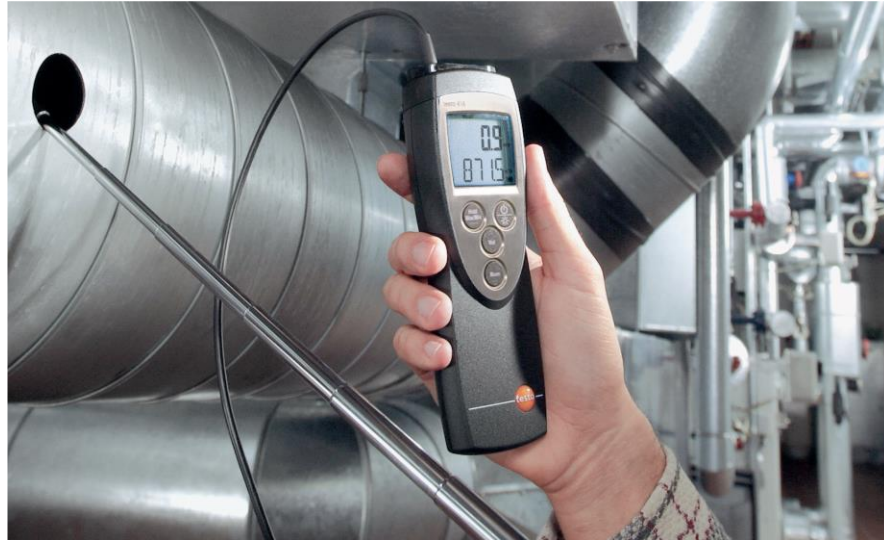
Fig. 4.21. Testo 405i thermoanemometer with telescopic probe
