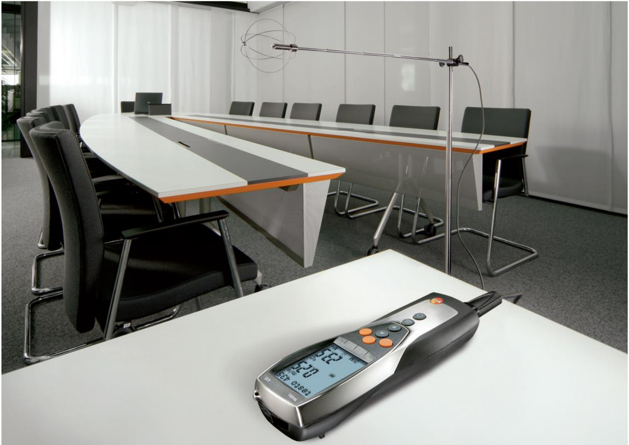
Fig. 4.25. Measuring comfort with the Testo 435 device
