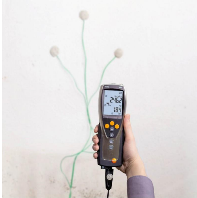
Fig. 5.17 Measuring wall surface temperature
